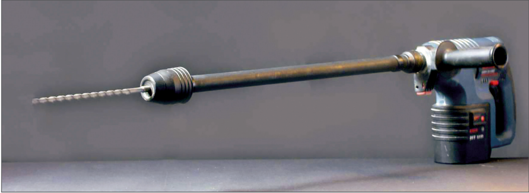
Battery drill, drill extension bar and SDS-drill
