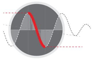
The above diagram shows a typical example of how PD measurement is carried out during the slope of the applied voltage. The steepness of the VLF CR and DAC slopes in comparison to the 0.1 Hz sine wave can be clearly seen.
