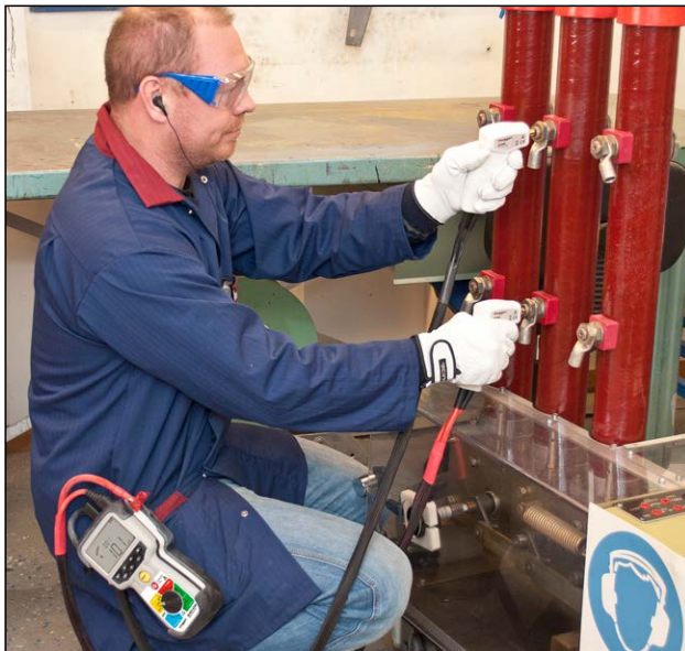
Hold probes / attach Kelvin clamps to CB and press trig / TEST button. A signal indicates whether test was pass or fail and result is logged in unit for later dump to PC.
